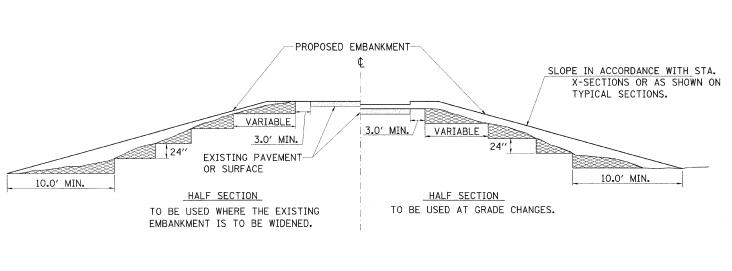
MATERIAL TO BE REMOVED AND REPLACED IN THE EMBANKMENT IN ACCORDANCE WITH ART. 205.04 OF THE STANDARD SPECIFICATION. COST TO BE INCLUDED IN THE VARIOUS ITEMS OF EXCAVATION AND NO ADDITIONAL COMPENSATION WILL BE ALLOWED BECAUSE OF THIS WORK.
