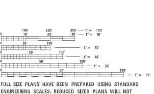
ENGINEERING SCALES, REDUCED SIZED PLANS WILL NOT CONFORM TO STANDARD SCALES. IN MAKING MEASUREMENTS ON REDUCED PLANS, THE ABOVE SCALES MAY BE USED.
