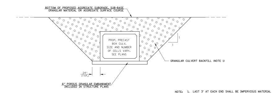
SECTION THROUGH PRECAST BOX CULVERT
