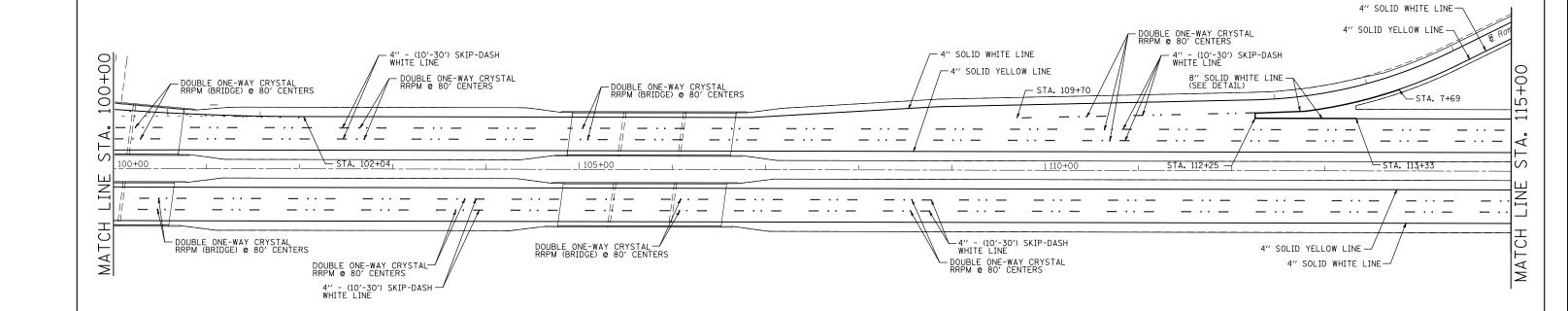
NOTE: ALL PAVEMENT MARKING ON STRUCTURES SHALL BE "PREFORMED PLASTIC PM, TYPE B" (WITH GROOVING), CONCRETE SURFACE ONLY.
