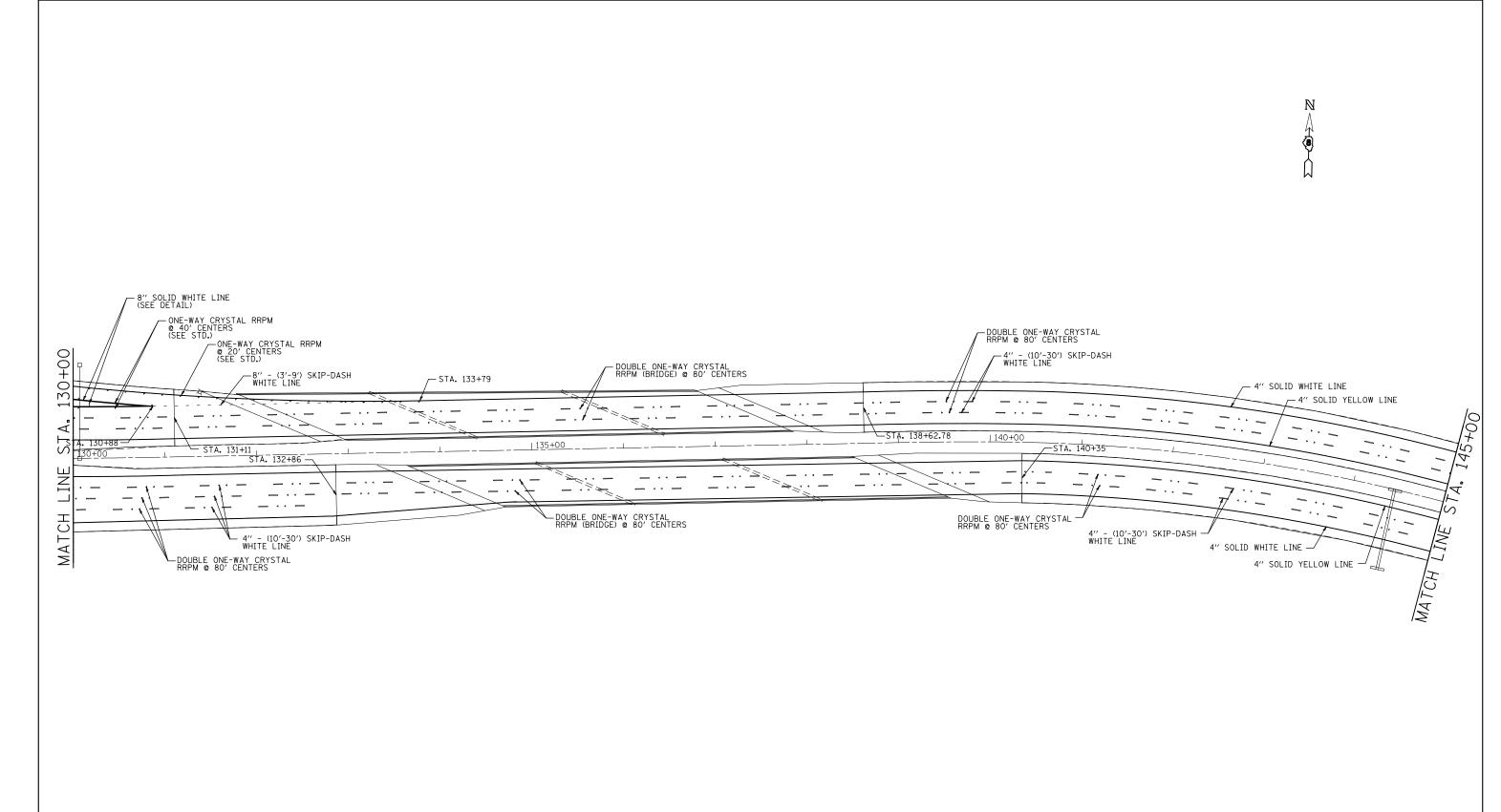
NOTE: ALL PAVEMENT MARKING ON STRUCTURES SHALL BE "PREFORMED PLASTIC PM, TYPE B" (WITH GROOVING), CONCRETE SURFACE ONLY.
