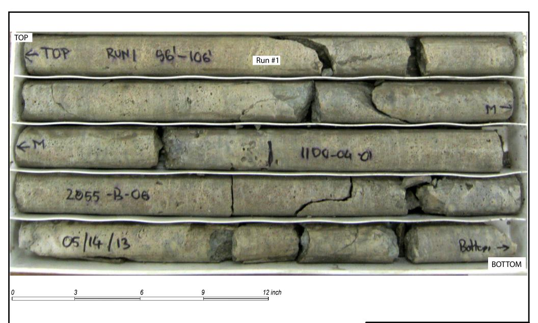
Boring 2055-B-06 Run #1, 96' to 106', RECOVERY = 97.5%, RQD = 71.67% ROCKCORE: CIRCLE INTERCHANGE RECONSTRUCTION, RETAINING WALL 38, SN 016-1827, CHICAGO, IL
