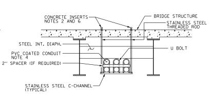
STAINLESS STEEL THREADED ROD BOTTOM-OF DECK CONCRETE INSERTS NOTES 2 AND 6 - STAINLESS STEEL NUTS, BOLTS, & WASHERS (TYPICAL)  $2^{1/2}$ " ×  $2^{1/2}$ " ×  $\frac{3}{16}$ PVC COATED CONDUITS NOTE 4
