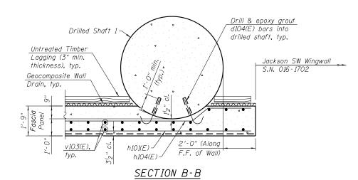
(Shaft reinforcement not shown for clarity)
