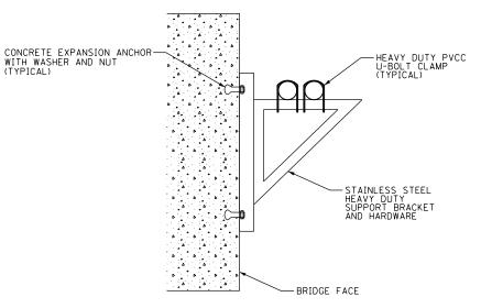
MOUNTING BRACKET FOR MULTIPLE CONDUITS NOT TO SCALE
