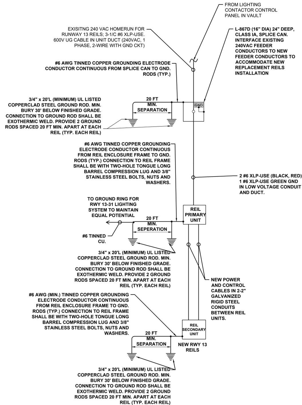
**PROPOSED ELECTRICAL ONE-LINE DIAGRAM FOR RWY 13 REILS**
