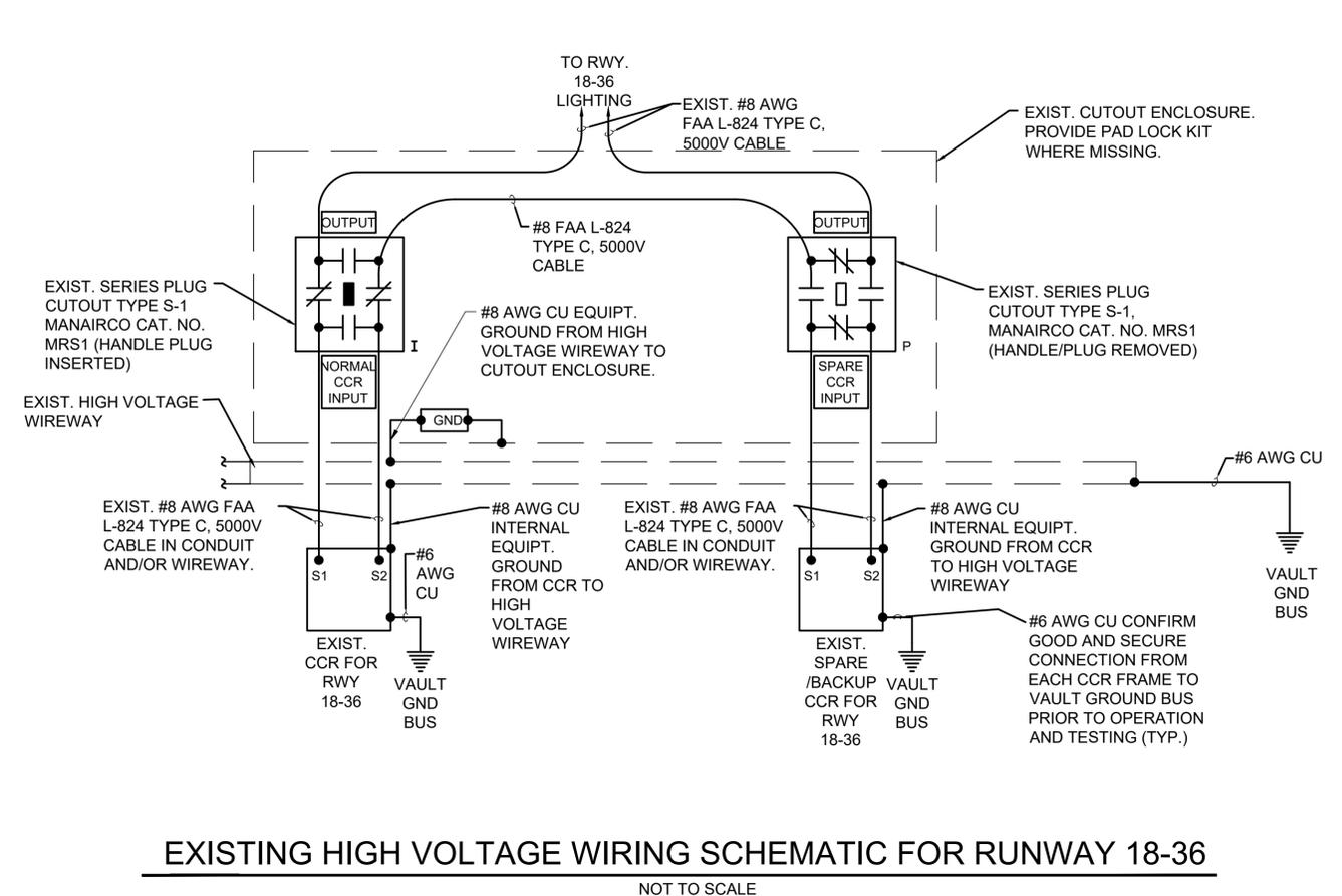
**EXISTING HIGH VOLTAGE WIRING SCHEMATIC FOR RUNWAY 18-36**
