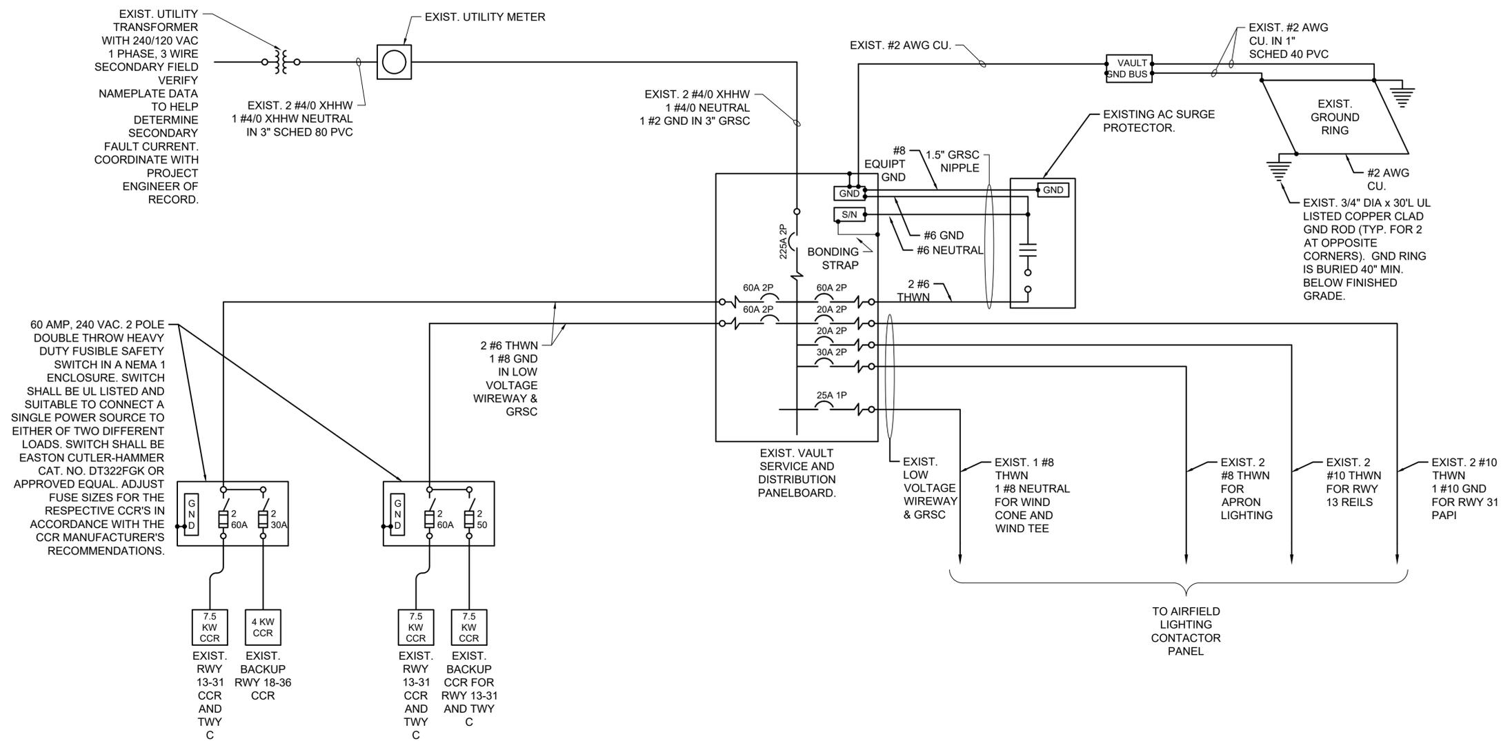
60 AMP, 240 VAC, 2 POLE DOUBLE THROW HEAVY DUTY FUSIBLE SAFETY SWITCH IN A NEMA 1 ENCLOSURE. SWITCH SHALL BE UL LISTED AND SUITABLE TO CONNECT A SINGLE POWER SOURCE TO EITHER OF TWO DIFFERENT LOADS. SWITCH SHALL BE EASTON CUTLER-HAMMER CAT. NO. DT322FGK OR APPROVED EQUAL. ADJUST FUSE SIZES FOR THE RESPECTIVE CCR'S IN ACCORDANCE WITH THE CCR MANUFACTURER'S RECOMMENDATIONS.
