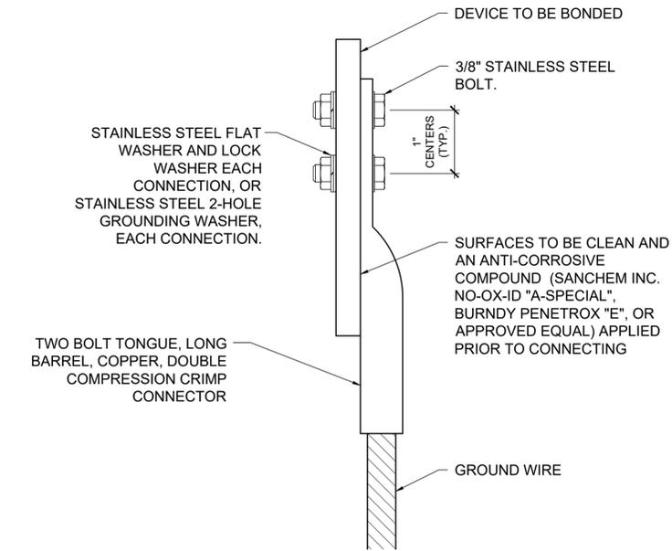
**2 HOLE LONG BARREL COMPRESSION LUG TABLE (OR APPROVED EQUAL)**
