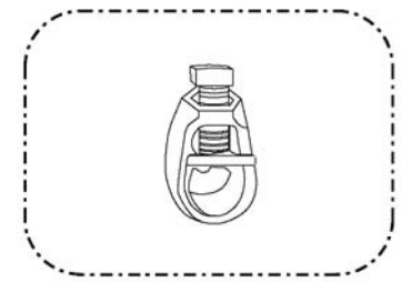
3/4" (20mm) HEAVY-DUTY GROUND ROD CLAMP (BURNDY TYPE GRC OR APPROVED EQUAL)
