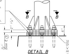
Ribs shall be cut to fit slope of pipe.
