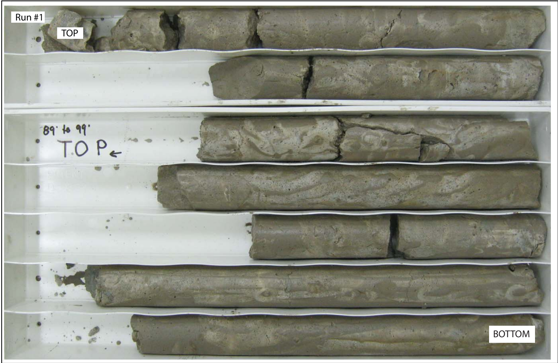
Boring 1087-B-02: Run #1, 89' to 99', RECOVERY = 100%, RQD = 84%
