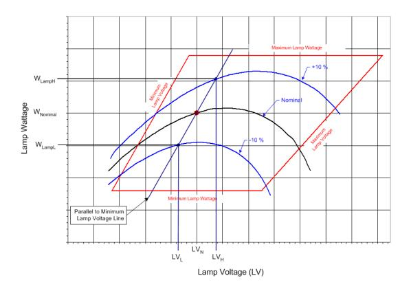
Ballast Regulation =  $\frac{W_{LampH} - W_{LampL}}{W_{LampN}} \times 100$
