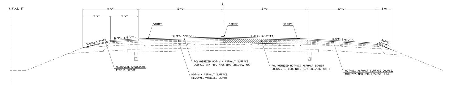
VARIABLE DEPTH HOT-MIX ASPHALT SURFACE REMOVAL IN PASSING LANE HOT-MIX ASPHALT SURFACE REMOVAL, 6" IN DRIVING LANE
