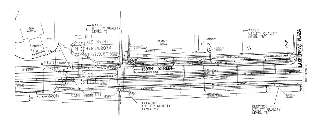
The SBC locations depicted have been obtained through the application of geophysical methods to determine the existence and approximate horizontal position of these facilities. However, SBC will not provide TBE Group, Inc. with utility records to help verify the locations of their existing underground facilities. Therefore, TBE is unable to verify the completeness of the SBC locations depicted in accordance with the CI/ASCE Standard 38-02.
