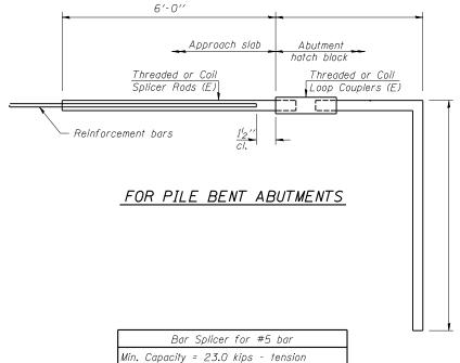
Min. Pull-out Strength = 9.2 kips - tension
