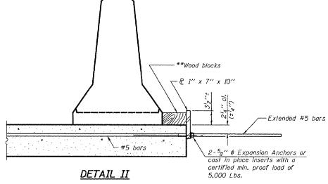
\*\* Wood blocks may be omitted when required to provide minimum stage traffic lane width. When the wood blocks are omitted, the concrete barrier shall be in direct contact with the steel retainer plate.
