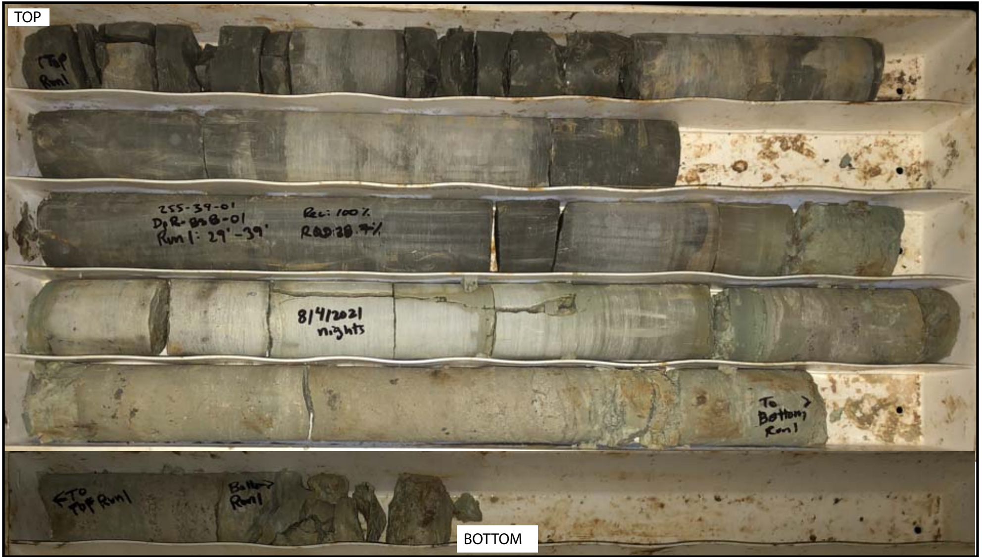
Boring DpR-BSB-01: Run #1, 29.0 to 39.0 feet, RECOVERY=100%, RQD=29%
