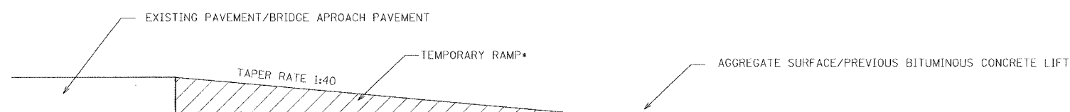
TEMPORARY RAMP DETAIL STAGE III CONSTRUCTION ONLY
