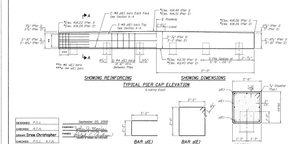
\*Elevations shown have been obtained from existing plans and are provided for <u>INFORMATION</u>
