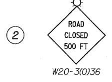
Post mounted sign with Type A Flashing Light
