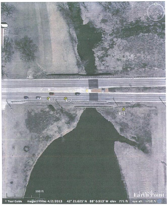
Boring Location Diagram Washington Street over Mill Creek-Wall Extension Midland Standard Engineering & Testing, Inc. MSET# 13299 August 2013 MIDLAND STANDARD ENGINEERING & TESTING, INC. STRUCTURE FOUNDATION BORING LOG
