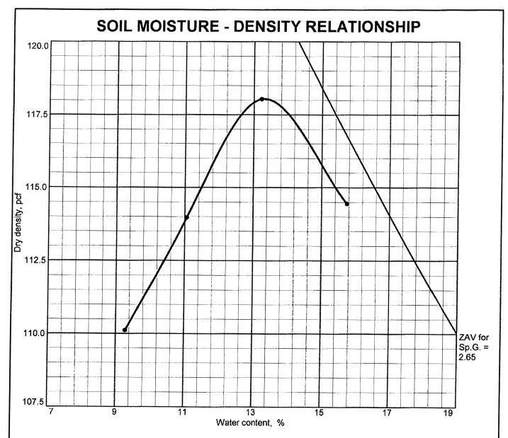
Test specification: ASTM D 698-00a Method A Standard
