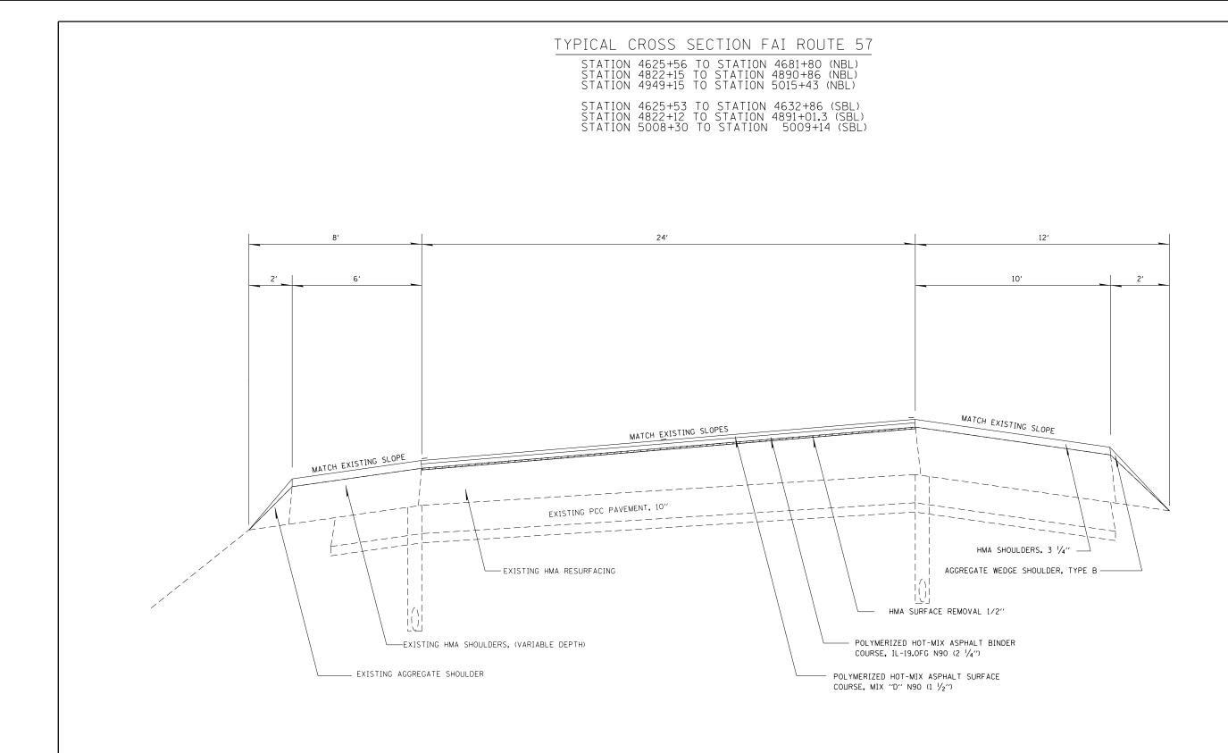
NOTE: THE MAXIMUM ALGEBRAIC DIFFERENCE BETWEEN PAVEMENT SLOPE AND SHOULDER SLOPE SHALL NOT EXCEED 8%.
