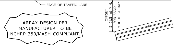
DETAIL "A" IMPACT ATTENUATOR, TEMPORARY (SEE NOTE 5)
