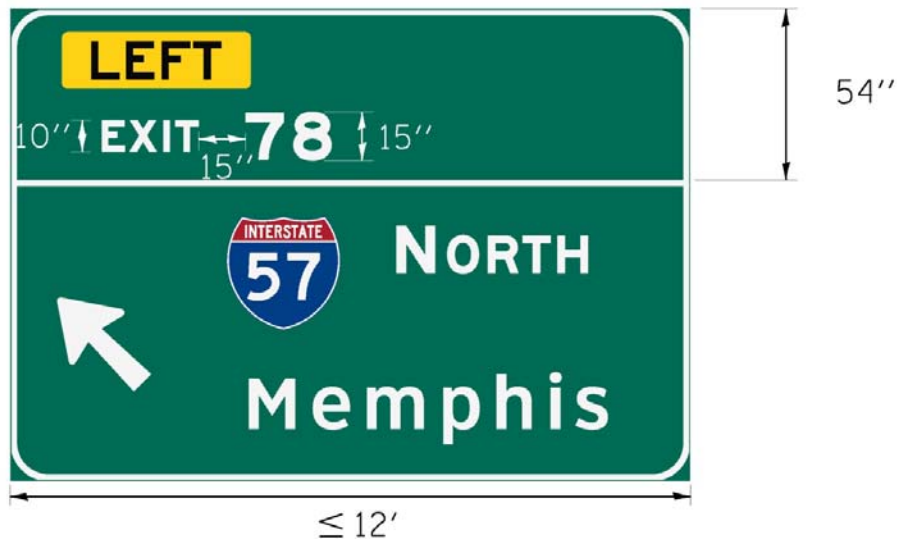
Figure 2M – Design of Left Exit Number Plaques for Sign Panels ≤ 12’ Wide
