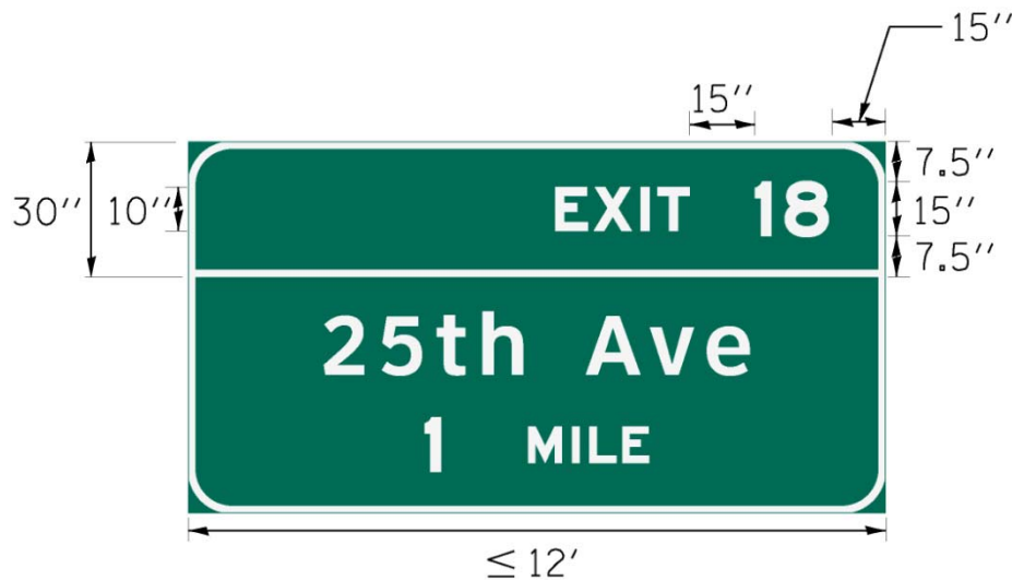
Figure 2M – Design of Left Exit Number Plaques for Sign Panels ≤ 12’ Wide
