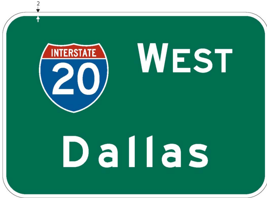
Figure 2A – Light borders on dark backgrounds shall have a 2 inch wide border
