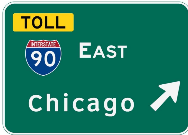
Figure 2V – Acceptable placement of supplemental “TOLL” plaque
