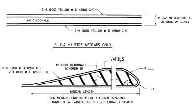
DIAGONAL LINE SPACING: 50' (15 m) C-C (LESS THAN 30MPH (50 km/h))
