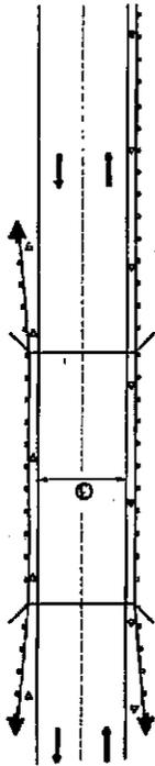
③ Bidirectional silver/amber should be used in lieu of monodirectional silver on both sides of two-lane bridges where the bridge pavement is less than 24 (610) wider than the pavement approaching the bridge.
