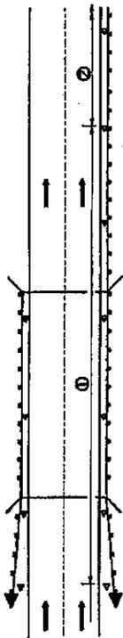
① Spacing 80 ft. (24 m) max. for first 400 ft. (122 m) or curve spacing shown in Standard 635001, whichever is less (min. 4 reflectors regardless of length).
