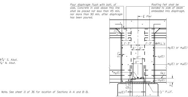
\* Tightly fasten the #8 bars together with No. 9 wire ties.
