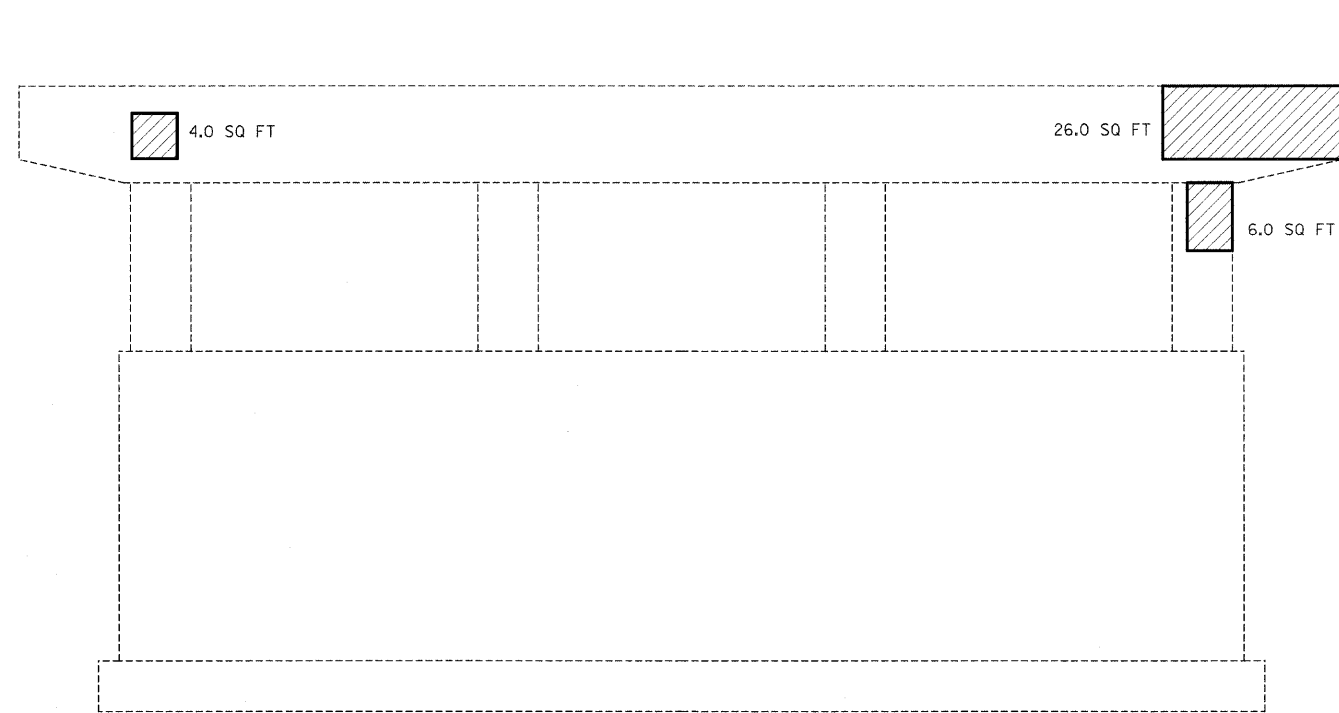
PIER #1 - WEST FACE
