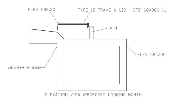
\*\* TYPE 15 FRAME & LID ADJUSTED TO PLAN HEIGHT USING MATERIALS AND METHODS APPROVED BY THE ENGINEER
