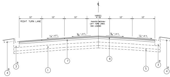
PROPOSED TYPICAL CROSS SECTION STA. 15+00 TO 16+19
