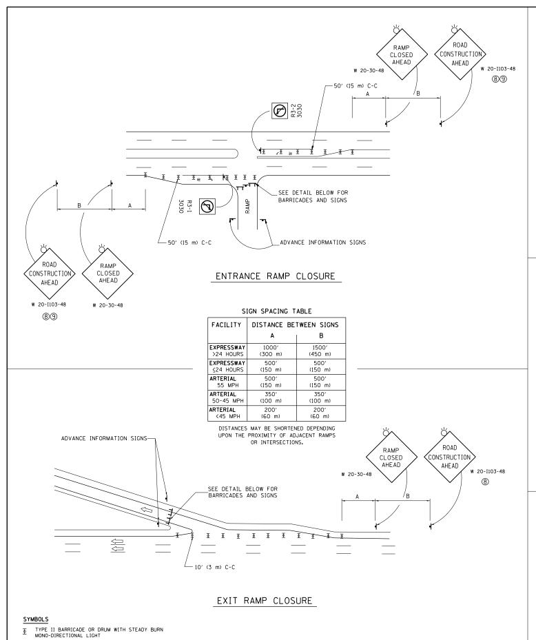
TYPE III BARRICADE WITH 2 FLASHING LIGHTS
