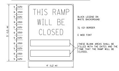
THESE SIGNS ARE REQUIRED ON BOTH SIDES OF THE RAMP, MINIMUM OF 1 WEEK IN ADVANCE OF THE CLOSURE.
