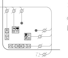
THE CONTRACTOR SHALL REPLACE THE EXISTING TRAFFIC SIGNAL POST WITH THE PROPOSED TRAFFIC SIGNAL POST, 14 FT. AND ATTACH THE PROPOSED POST TO THE EXISTING FOUNDATION.
