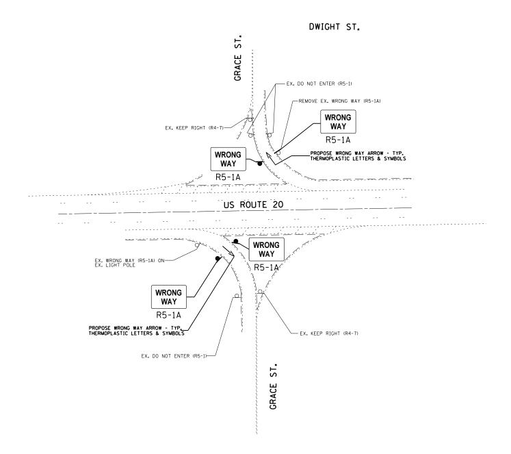
NOTE: SIGN ASSEMBLIES GREATER THAN 16 SOUARE FEET REOUIRE 2 TELESCOPING STEEL SIGN SUPPORTS.
