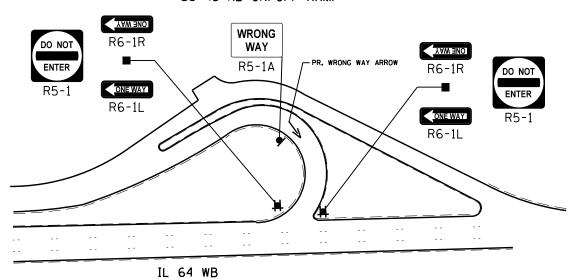
NOTE: SIGN ASSEMBLIES GREATER THAN 16 SQUARE FEET REQUIRE TWO TELESCOPING STEEL SIGN SUPPORTS.
