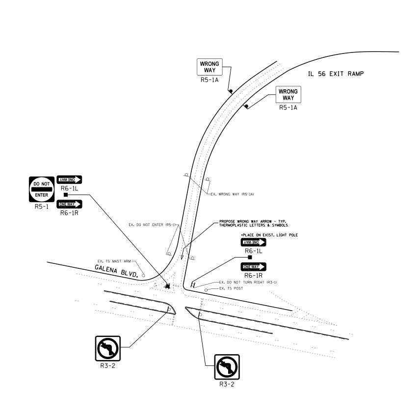
NOTE: SIGN ASSEMBLIES GREATER THAN 16 SOUARE FEET REQUIRE 2 TELESCOPING STEEL SIGN SUPPORTS.
