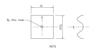
Plate A shall be placed between rall element and block-out at non-splice mounting points only when steel block-outs are used.
