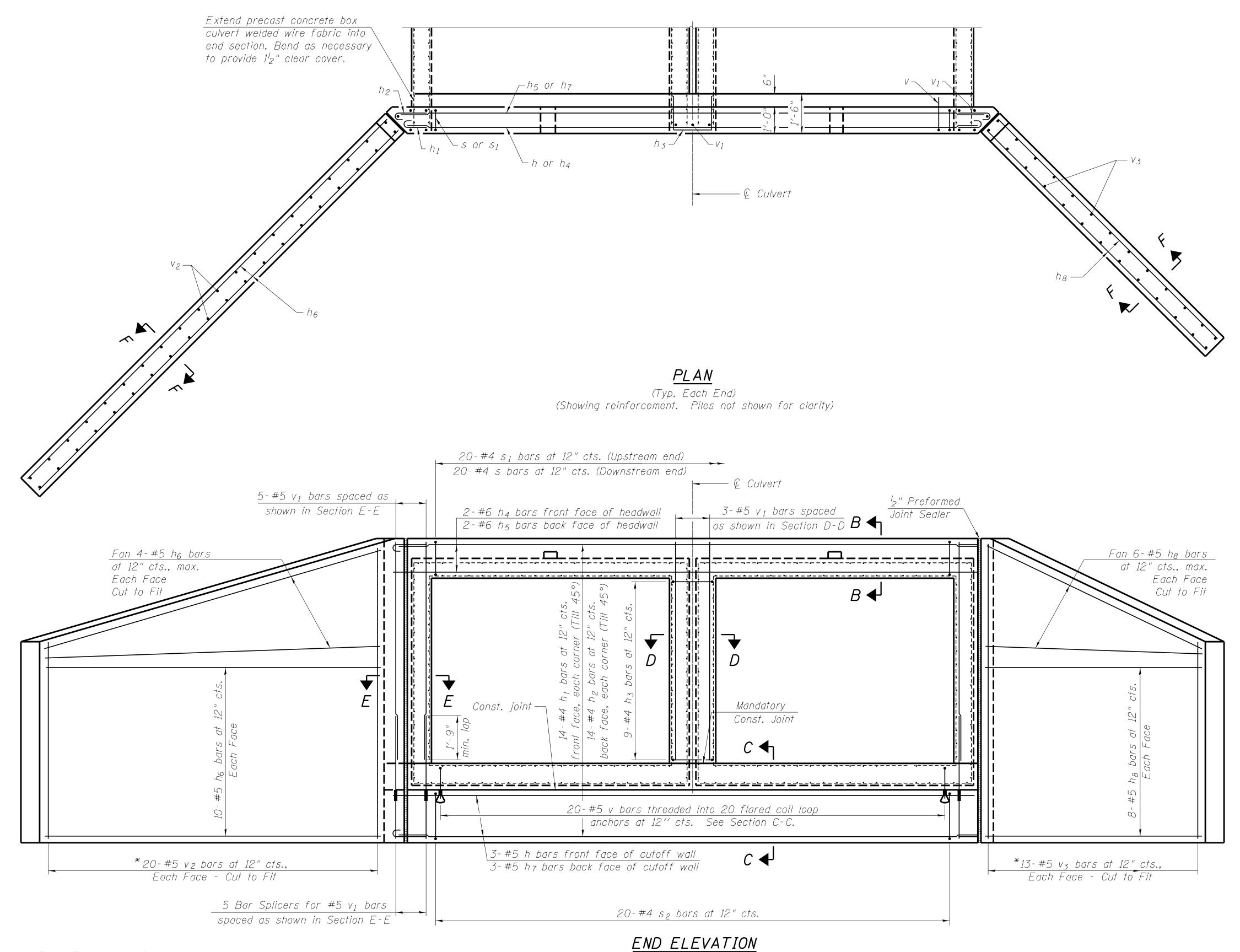
\* See sheet 4 of 7 for Field Cutting Diagram..
