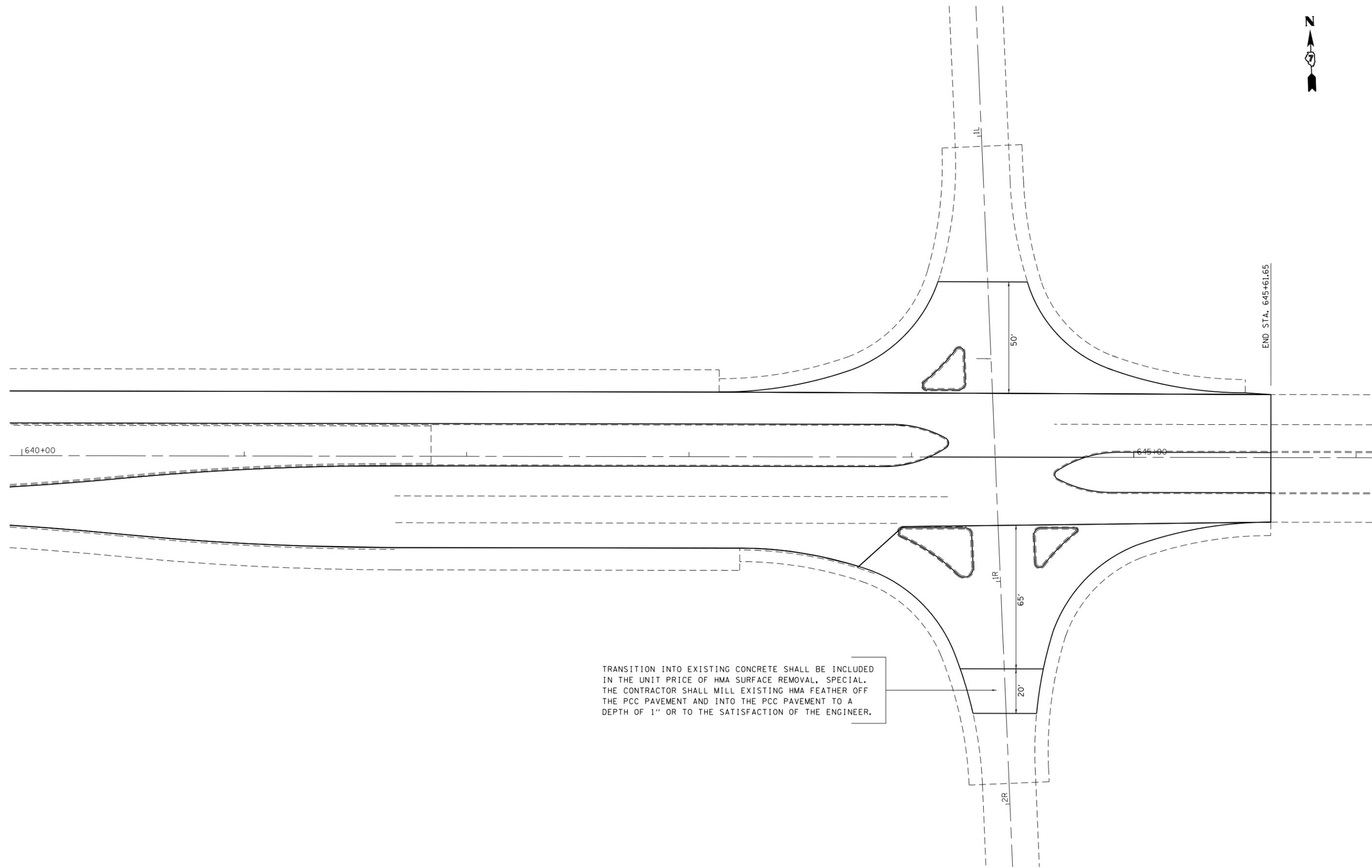
TRANSITION INTO EXISTING CONCRETE SHALL BE INCLUDED IN THE UNIT PRICE OF HMA SURFACE REMOVAL, SPECIAL. THE CONTRACTOR SHALL MILL EXISTING HMA FEATHER OFF THE PCC PAVEMENT AND INTO THE PCC PAVEMENT TO A DEPTH OF 1" OR TO THE SATISFACTION OF THE ENGINEER.
