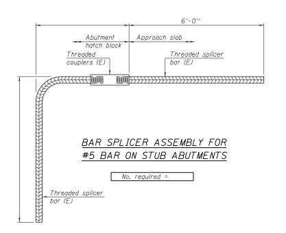
Splicer bars shall be deformed with threaded ends and have a minimum 60 ksi yield strength.
