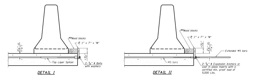
•• Wood blocks may be omitted when required to provide minimum stage traffic lane width. When the wood blocks are omitted, the concrete barrier shall be in direct contact with the steel retainer plate.
