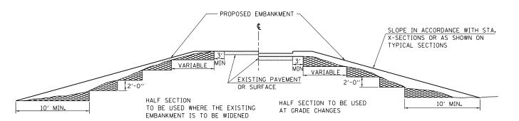
MATERIAL TO BE REMOVED AND REPLACED IN THE EMBANKMENT IN ACCORDANCE WITH ART. 205.04 OF THE STANDARD SPECIFICATION. COST TO BE INCLUDED IN THE VARIOUS ITEMS OF EXCAVATION AND NO ADDITIONAL COMPENSATION WILL BE ALLOWED BECAUSE OF THIS WORK.
