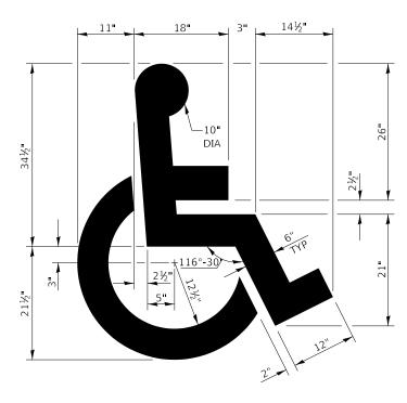
TYPICAL DETAIL FOR PAINTING HANDICAP MARKINGS
