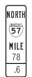
TYPICAL ENHANCED REFERENCE LOCATION SIGN (SEE SIGNING SCHEDULE AND MILE POST MARKER SIGN SCHEDULE FOR LOCATIONS)
