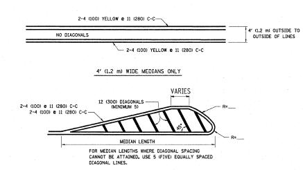
DIAGONAL LINE SPACING: 50' (15 m) C-C (LESS THAN 30MPH (50 km/h)) 75' (25 m) C-C 30MPH (50 km/h) TO 45MPH (70 km/h)) 150' (45 m) C-C (MORE THAN 45MPH (70 km/h))
