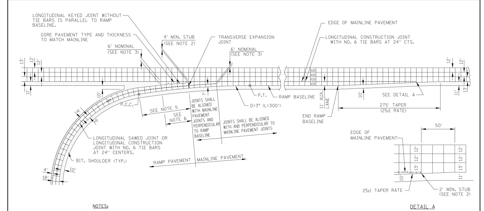
1. ALL PAVEMENT JOINTS SHALL BE DETAILED AS SHOWN ON I.D.O.T. HWY. STANDARD 420001, EXCEPT EXPANSION JOINT SEALS SHALL BE AS DESCRIBED IN THE SPECIAL PROVISION, BONDED PREFORMED JOINT SEALER.
