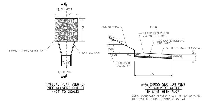
PIPE CULVERT OUTLET DETAIL
