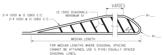
DIAGONAL LINE SPACING: 50' (15 m) C-C (LESS THAN 30MPH (50 km/h))
