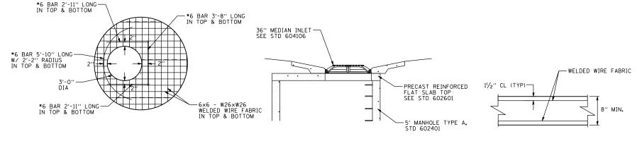
5' FLAT SLAB TOP DETAIL WITH 36" OPENING
