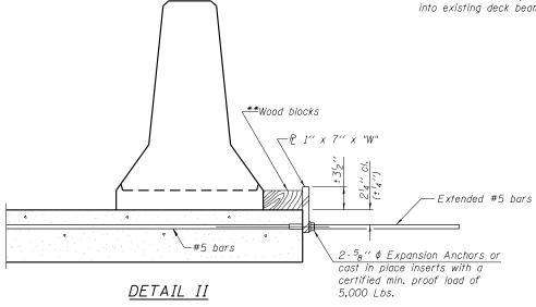
Top bars - Detail I spacing - Detail II  $-\mathcal{Q}^{7}_{8}^{\prime\prime}$  \$\phi\$ Holes \*£ 1" x 1'2" Notch
