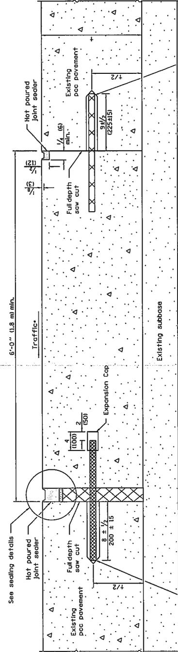
18 (450) Long dowel bars anchored into existing pavement at 12 (300) cts.
