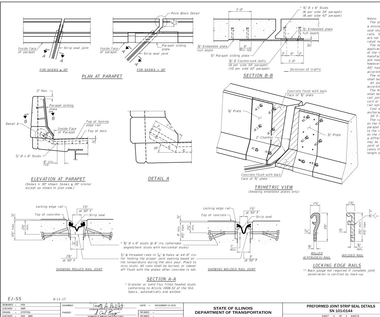
The strip seal shall be made continuous and shall have a minimum thickness of  $\frac{1}{4}$ ". The configuration of the strip seal shall match the configuration of the locking edge rails. Open or "webbed" strip seal gland configurations are not permitted. The gland shall be sized for a maximum rated movement of 4 inches.
